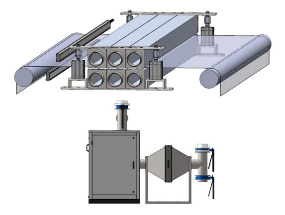
The air flow unit (AFU), housed in a compact foot mounted enclosure, provides the necessary air delivery and suction to the web cleaning station.
